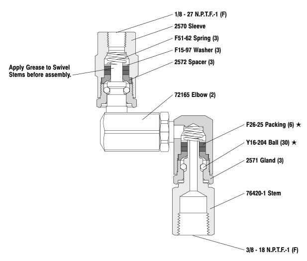
★ Parts so Marked are Included in 61239 Repair Kit.
